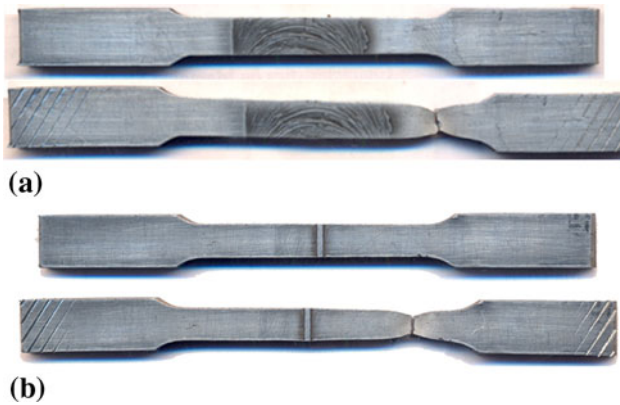
Fig. 7 Fracture location of tensile specimens. (a) FSW and (b) LBW
